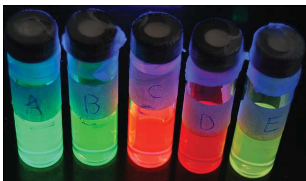
Figure 4 Fluorescent electrospinning solutions containing QDs with fluorescence peaks at (A) 525 nm QDs, (B) 550 nm, (C) 590 nm, (D) 615 nm and (E) 525 and 615 nm. [Color figure can be viewed in the online issue, which is available at wileyonlinelibrary.com .]
